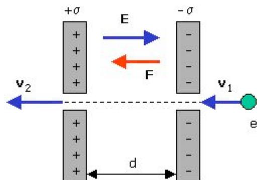
$$L = \Delta E_c = \frac{1}{2} m v_2^2 - \frac{1}{2} m v_1^2 = \frac{1}{2} m \cdot (v_2^2 - v_1^2) = \frac{1}{2} \cdot 9,1 \cdot 10^{-31} \cdot [(9,0 \cdot 10^5)^2 - (1,0 \cdot 10^5)^2] = 364 \cdot 10^{-21} \text{ J}$$
